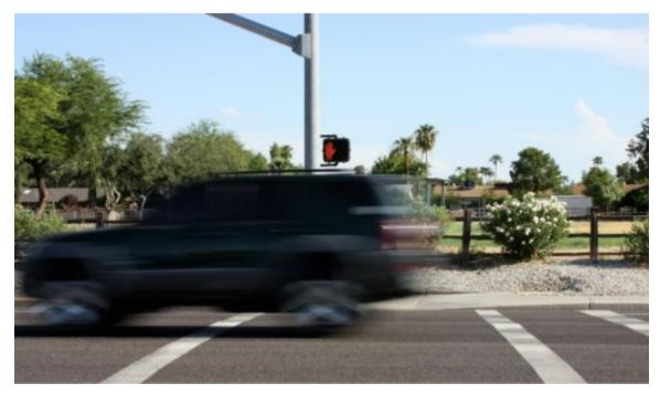
The photo above was taken with the camera shutter open for 1/20 sec. The distance between white stripes is 3 meters. The length of the blur is the distance the car traveled while the shutter was open.
